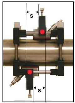
Figure 3-12: Top View of V4 Fixture with Both Transducers
